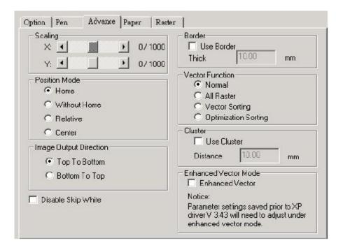
In this panel, you want to leave the scaling off, POSITION MODE should be home (this tells the Laser Cutter to start at 0,0 and cut as you have it drawn on the page). Make sure the BORDER is unchecked, and the VECTOR FUNCTION is set to VECTOR SORTING (this will cut the inside parts out first, which is good because the part will drop otherwise). Keep everything else unchecked.
